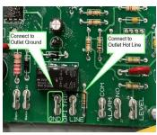
• **GFCI Trip**: By connecting a wire from the GFCI GND Tab to the Ground of an outlet, and wire from the LINE Tab to the Hot Wire of the outlet when the alarm sounds for 5 seconds, a pulse is issued to trip the GFCI breaker that is associated with that outlet. Test the GFCI tripping by pressing and holding the TEST button for 5 seconds. Warning: Wires should be in conduit.
