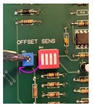
• Zero Reference Point: In bodies of water that have a very high Ambient Voltage in the water (i.e. 2 Volts+), The default zero reference point can be adjusted to the current environment. Default setting is 0 Volts. By turning this pot clockwise reference point will be increased which can be seen by the number of LEDs being displayed decreasing. With this feature you can set up the system to alarm at "X" Volts over ambient voltage.
