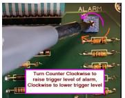
• Alarm Trigger Point: The Alarm is set to trigger off the number of LEDs lit (not voltage). Factory default is usually between 2 and three yellow LEDs. Alarm level can be raised by turning the Alarm pot counter clockwise. Example: Sensitivity dip switch is set to 1 up (0.25 Volts) and alarm is set to trigger on the  $6^{th}$  LED, which corresponds to (0.25 \* 6 = 1.5 Volts).
