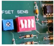
**Sensitivity Settings**: Internal dip switches allow for increasing the sensitivity level of the unit. Increasing sensitivity increases range of detection. Factory Defaults is one switch up (0.25 Volts/LED) 0 = 0.5 Volts, 1 = 0.25 Volts, 2 = 0.16 Volts, 3 = 0.12 Volts, 4 = 0.08 Volts
