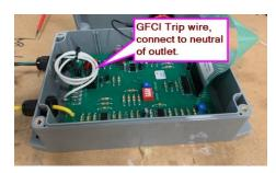
• **GFCI Trip**: By connecting this wire to the neutral of an outlet, when the alarm sounds it will send a pulse to trip the GFCI breaker that is associated with that outlet. It is recommended to use the battery backup option of the Dock Lifeguard to keep continuous power to the unit. Refer to users guide for more details.
