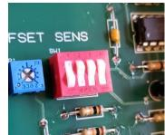
Sensitivity Settings: Internal dip switches allow for increasing the sensitivity level of the unit. Increasing sensitivity increases range of detection. Factory Defaults is one switch up (0.25 Volts/LED) 0 = 0.5 Volts, 1 = 0.25 Volts, 2 = 0.16 Volts, 3 = 0.12 Volts, 4 = 0.08 Volts
