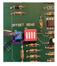
• Alarm Trigger Point: The Alarm is set to trigger off the number of LEDs lit (not voltage). Factory default is usually between 2 and three yellow LEDs. Alarm level can be raised by turning the Alarm pot counter clockwise. Example: Sensitivity dip switch is set to 1 up (0.25 Volts) and alarm is set to trigger on the 6<sup>th</sup> LED, which corresponds to (0.25 \* 6 = 1.5 Volts).
