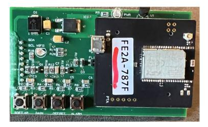
Align pins on the back of the DLG iOT board to the socket on the left side off the mother board and firmly push the board onto the mother board. There will be white plastic guide pin on the board that needs to be seated in the center hole of the mother board.
