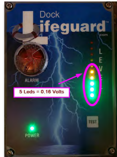
Four Switches in On (up) Position, each LED = 0.08 Volts
