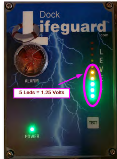
One Switch in On (up) Position, each LED = 0.25 Volts
