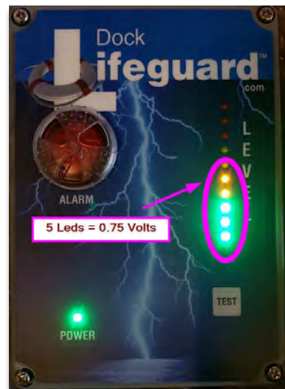
Two Switches in On (up) Position, each LED = 0.16 Volts
