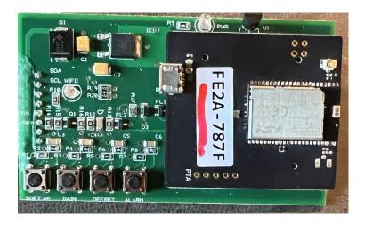
Align pins on the back of the DLG iOT board to the socket on the left side of the mother board and firmly push the board onto the mother board. There will be white plastic guide pin on the board that needs to be seated in the center hole of the mother board.
