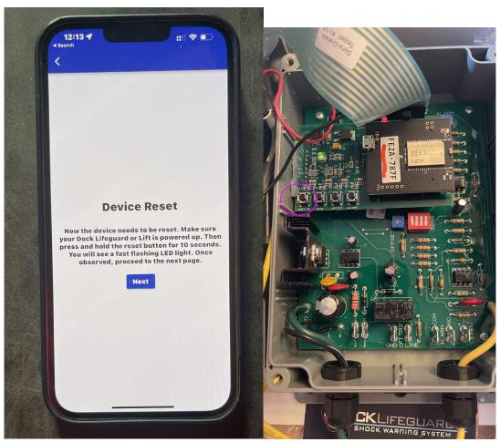
The reset button on the iOT board is labeled "SOFT AP"
